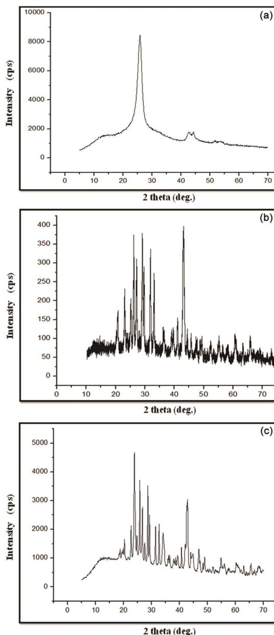
Fig. 2 – (a) XRD pattern of MWCNT, (b) XRD pattern of brine sludge and (c) XRD pattern of developed advanced material.
