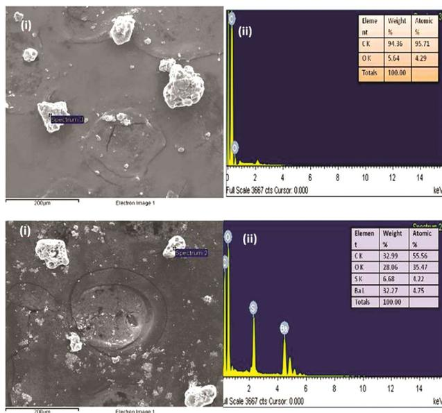
Fig. 5 – (a) EDXA image of (i) MWCNT (ii) EDXA outcomes and elemental compositions (weight% and atomic%) and (b) EDXA image of (i) synthesized advanced material (ii) EDXA outcomes and Elemental compositions (weight% and atomic%).
