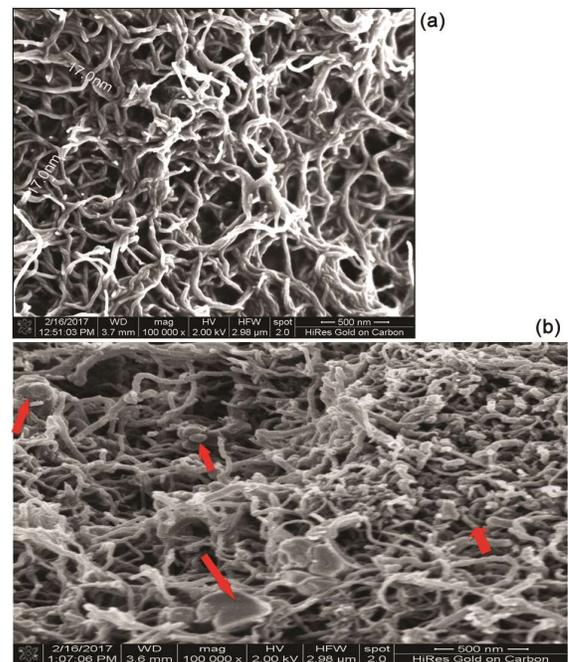
Fig. 4 – (a) FESEM image of MWCNTs and (b) FESEM image of developed advanced material.
