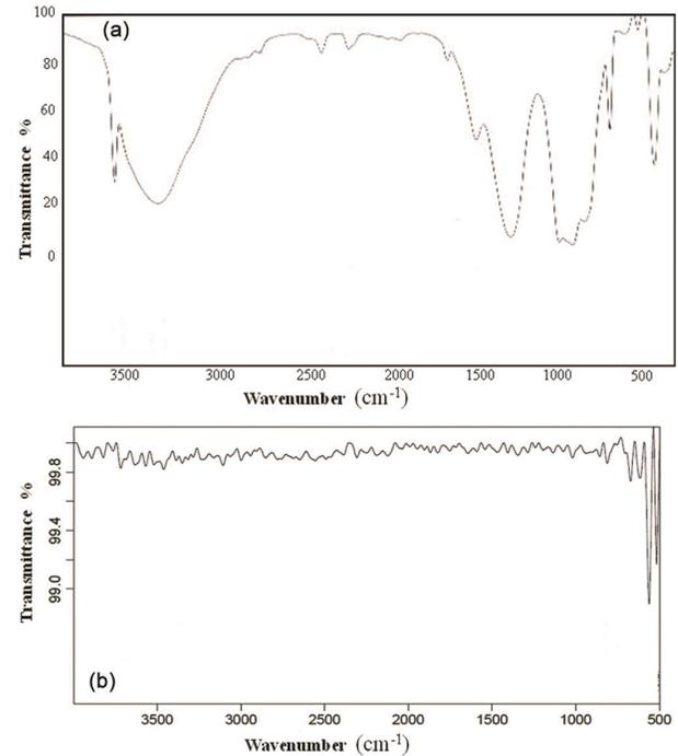
Fig. 3 – (a) FTIR spectrum of spectrum of brine sludge and (b) FTIR spectrum of spectrum of the developed advanced material.
