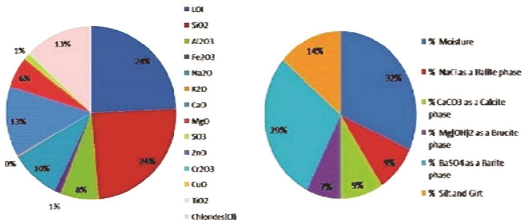
Fig. 1 – Mineralogical behaviour and chemical analysis of brine sludge.
