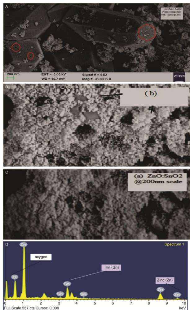
Fig. 5 — (A) SEM image for ZnO: SnO 2 (A) Nano rods; (B) Nanocomposite cluster (porous nature foams observed); (C) Images from SEM at 200 nm 100 k X times magnified ZnO:SnO 2 Nanocomposite clusters; and (D) EDS spectral Images confirms Zn, Sn, Oxygen Elements
