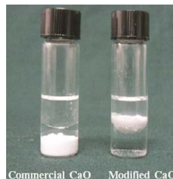
Fig. 2 — Dispersion of CaO particles in the methanol phase (lower) and rapeseed oil phase (upper) before and after modifying
