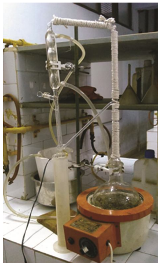
Fig. 1 – Experimental setup for extraction of patchouli oil
