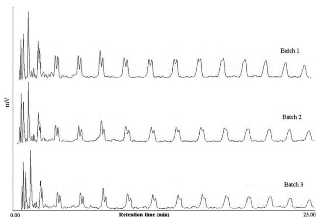
Fig. 5 — Gas chromatography characteristics of pyrolysis oil obtained at 500°C in three different batches batch-1, batch-2 and batch-3.
