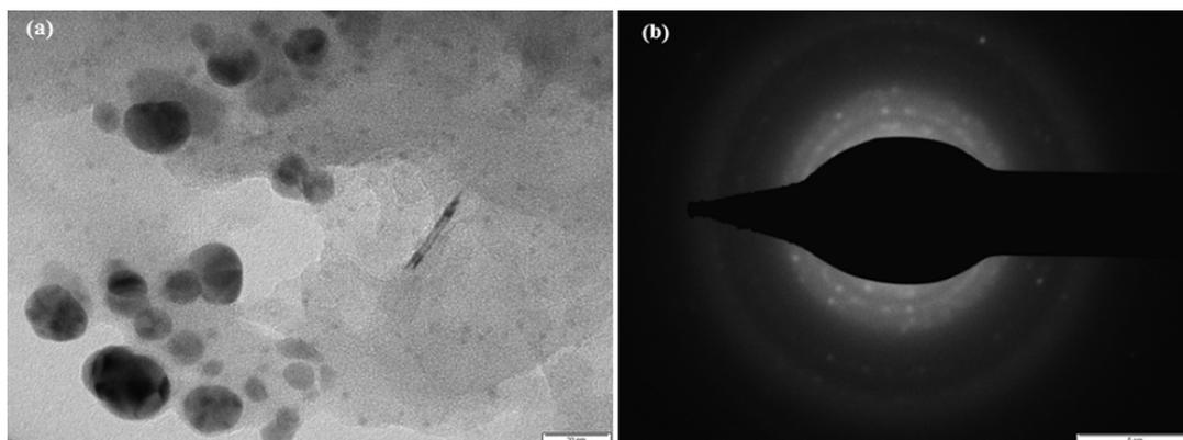
Fig. 1— (a-b) TEM and SAED pattern of the synthesized CuNPs.
