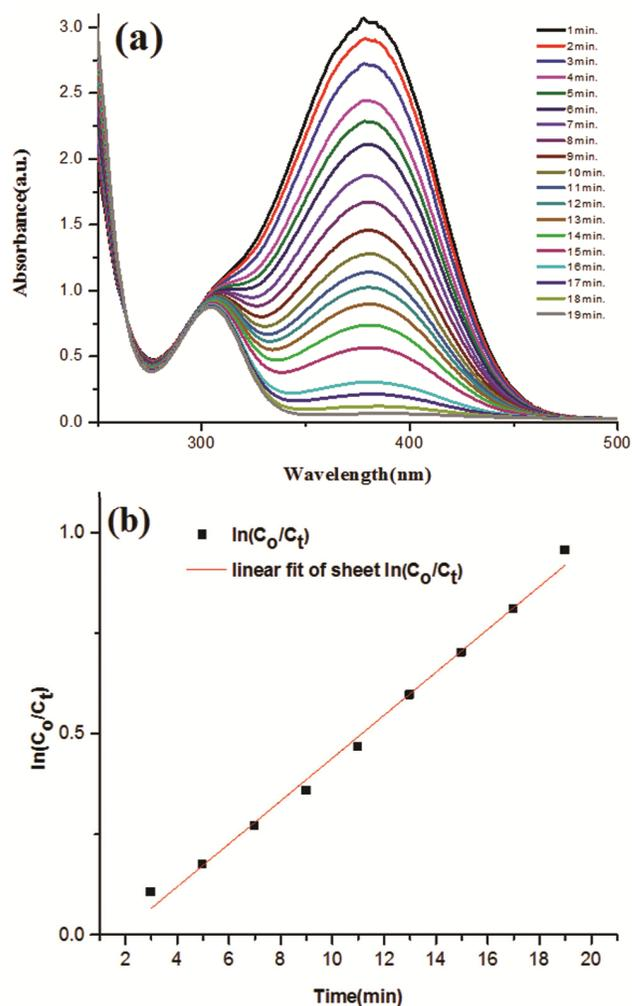
Fig. 4 — (a-b) Absorption spectra of reduction of para-nitroaniline using CuNPs as a catalyst in presence of NaBH<sub>4</sub> in aqueous medium and plot of  $\ln [C_0/C_t]$  versus reduction time.
