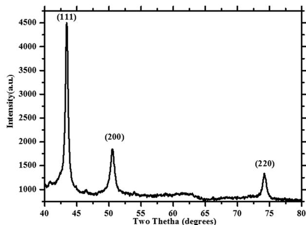
Fig. 2 — XRD peaks of the synthesized CuNPs.
