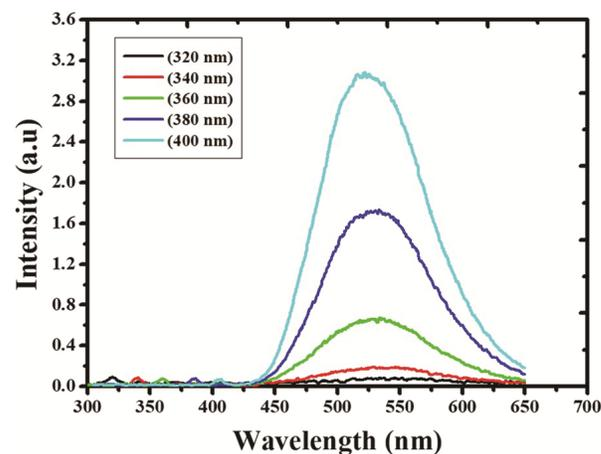
Fig. 2 — Fluorescence spectra (excited at 320 to 400 nm) of C-dot nanofillers.
