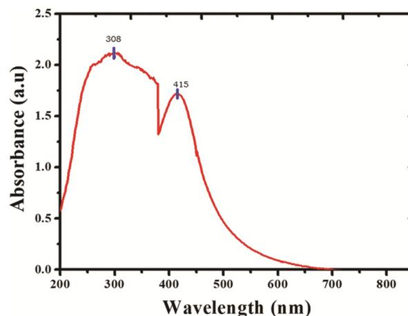
Fig. 1 — UV-Visible spectrum of the C-dot nanofillers.
