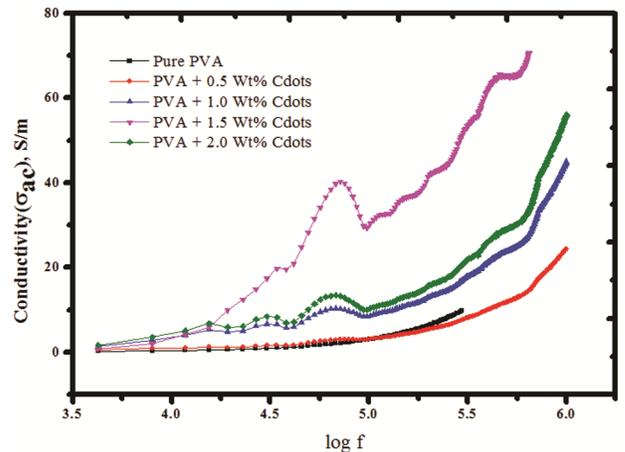
Fig. 7 — AC Conductivity of C-dot nanofiller PVA composite films as a function of log frequency
