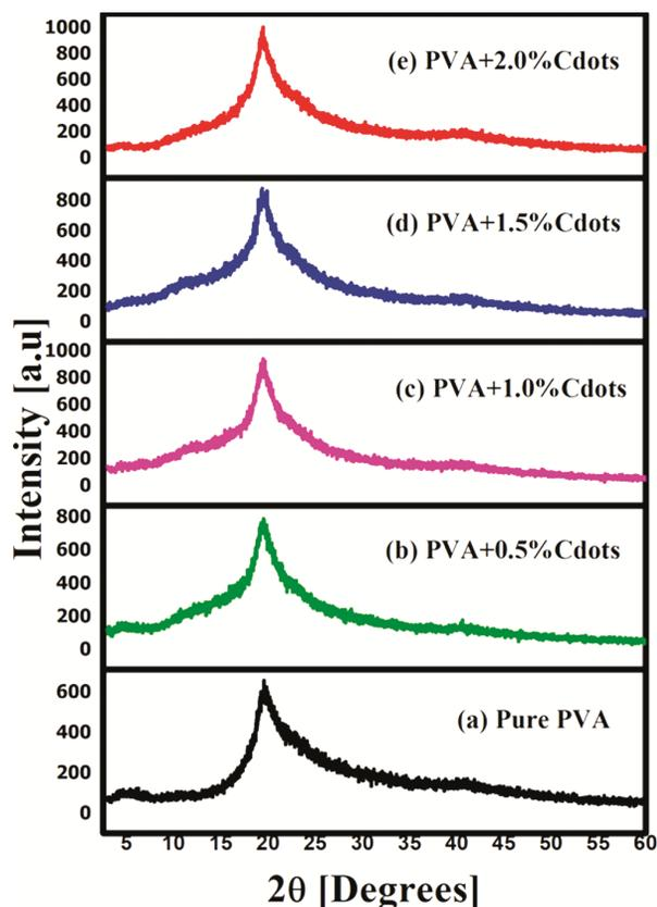
Fig. 4 — XRD profiles for a) 0wt % b) 0.5wt% c) 1wt% d) 1.5wt% e) 2wt% C-dot nanofiller loaded PVA composites
