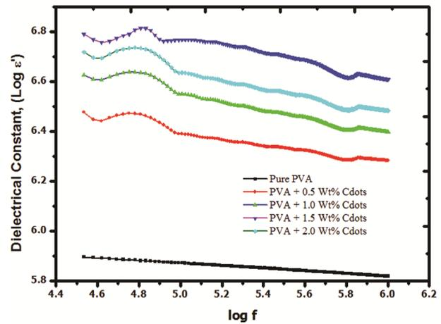
Fig. 6 — Dielectric constant of PVA–C-dot nanocomposites as a function of log frequency
