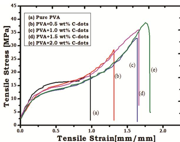
Fig. 5 — Stress-Strain diagram for (a) pristine PVA (b) 0.5wt% (c) 1wt% (d) 1.5wt% (e) 2wt% of C-dot nanofiller loaded in PVA matrix.
