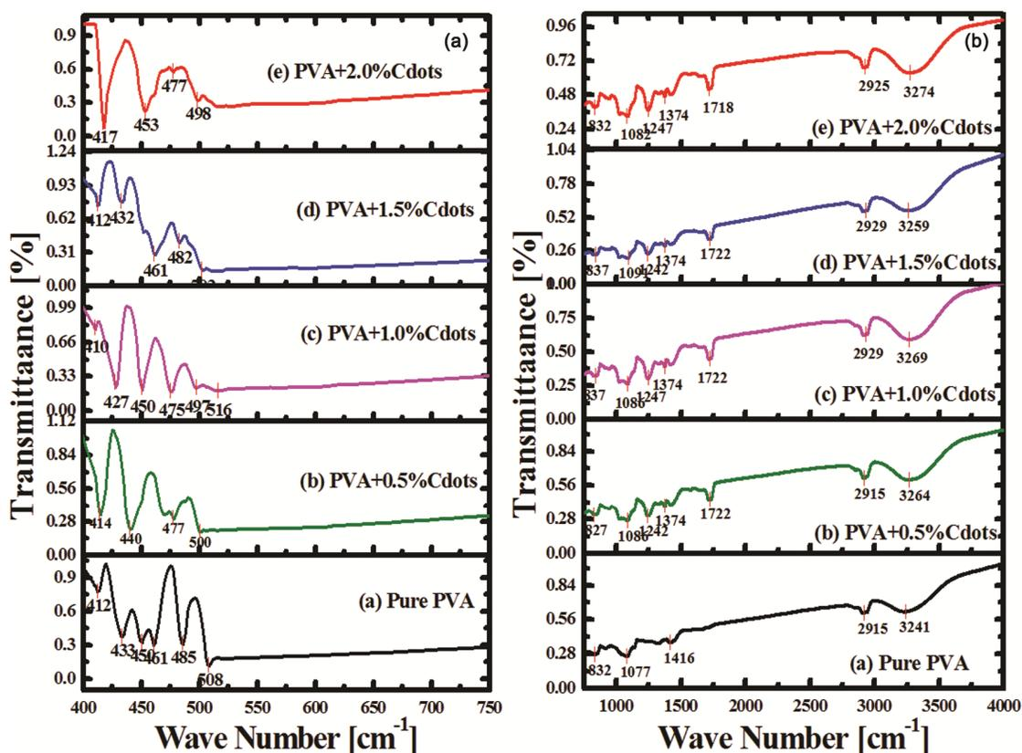
Fig. 3 — FTIR spectra for C-dot nanofiller PVA composite films from wavelength (a) 400 to 750 $\text{cm}^{-1}$  (b) 750 to 4000 $\text{cm}^{-1}$
