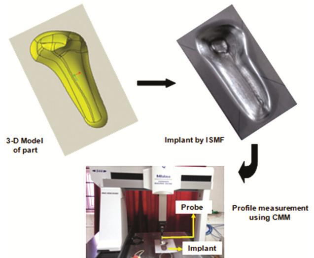
Fig.10 — Measurement and evaluation of formed knee part.
