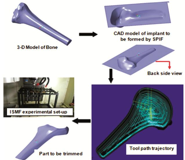
Fig. 7 — Fabrication steps involved in SPIF process.
