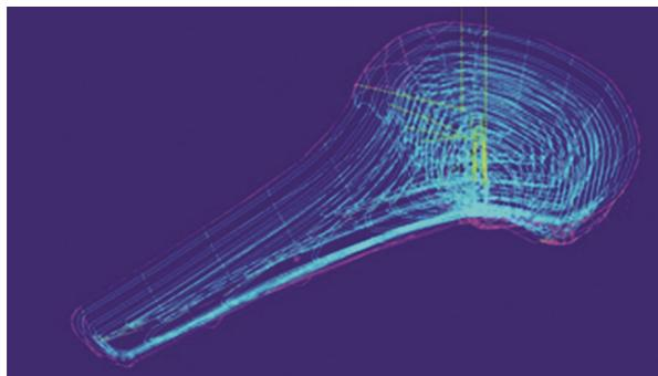
Fig. 3 — Tool path trajectory of knee implant.
