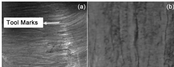
Fig. 12 — Surface examination of part (a) Hemispherical rigid tool, (b) Roller ball tool.
