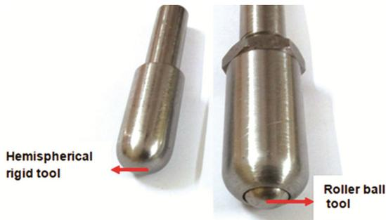
Fig. 6 — Profile of the forming tools.
