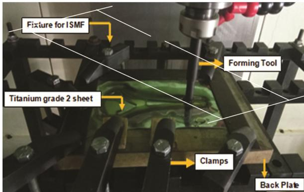
Fig. 5 — Experimental setup of SPIF on Ti grade 2 sheet.
