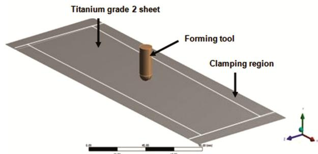
Fig. 4 — Assembly of sheet metal and forming tool geometry for finite element analysis.
