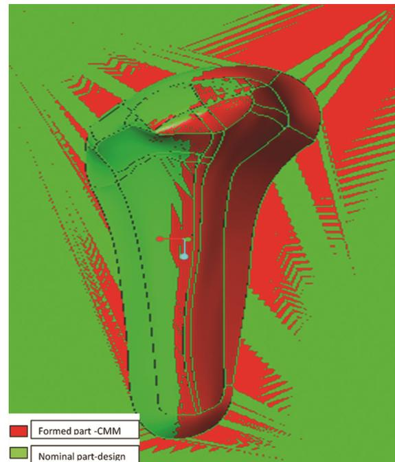
Fig. 11 — Comparison of the formed part with nominal design.
