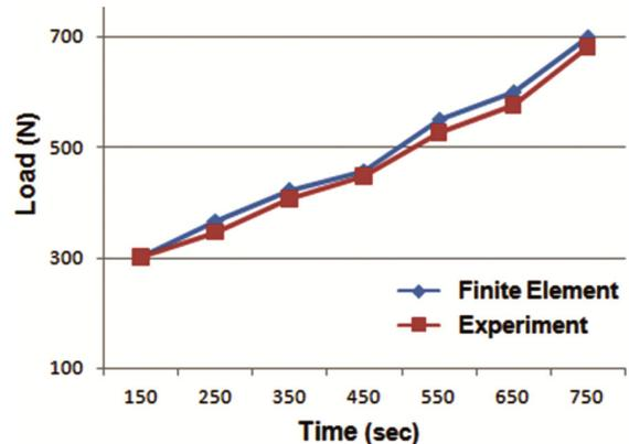
Fig. 8 — Forming load comparison.
