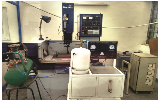
Fig. 1 — Developed experimental setup for PMND-EDM.
