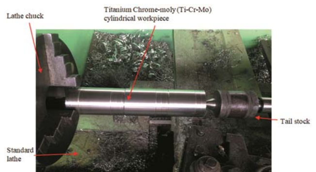
Fig. 1 — Experimental setup for turning the titanium chrome-molybdenum (Ti-Cr-Mo) cylindrical workpiece.
