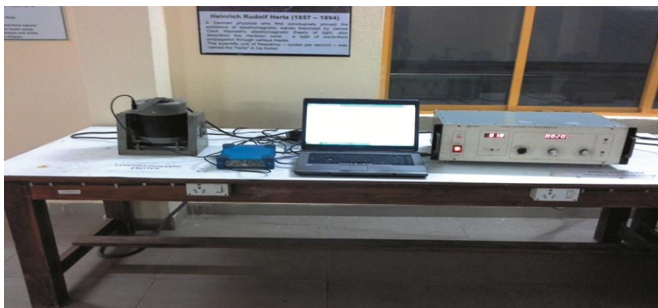
Fig. 1 — Setup for vibration test for carbon fibre beams.
