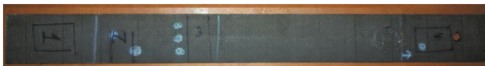
Fig 3 — White spot are small delamination area detected by ultrasonic test and numbers are marked for XRD analysis.
