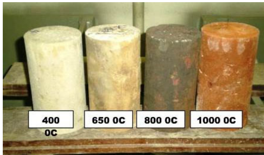
Fig. 5 — Appearance of geopolymer concrete after heat application at different temperature 48 .
