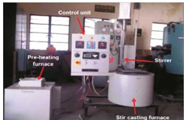
Fig. 1 — Stir casting unit along with control unit.
