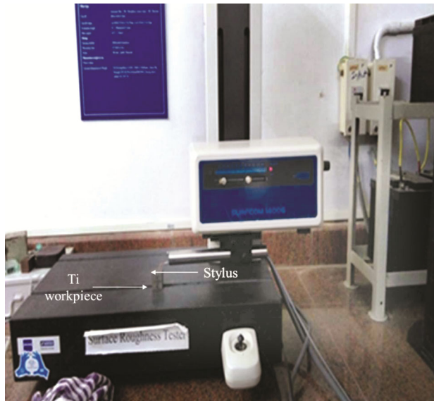
Fig. 3 — Surface roughness measurement setup.
