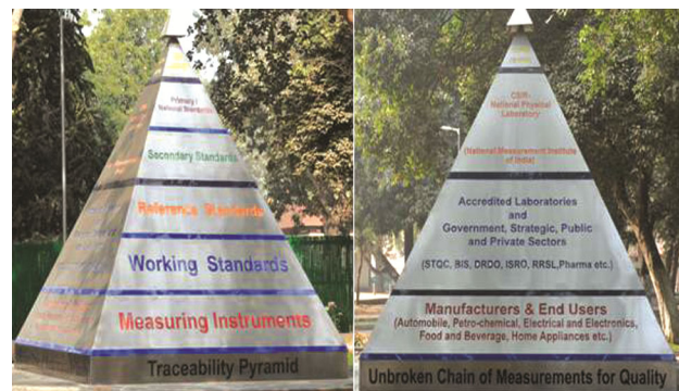
Fig. 1 — (a) Traceability pyramid of measurements and (b) Unbroken chain of measurements for quality.
