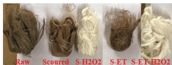
Fig. 6 — Raw, scoured, scoured-hydrogen peroxide bleached (S-H 2 O 2 ), scoured-enzyme treated (S-ET), and scoured-enzyme treated- hydrogen peroxide bleached (S-ET-H 2 O 2 ) jute fibres
