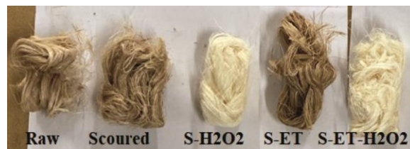
Fig. 7 — Raw, scoured, scoured-hydrogen peroxide bleached (S-H 2 O 2 ), scoured-enzyme treated (S-ET), and scoured-enzyme treated- hydrogen peroxide bleached (S-ET-H 2 O 2 ) banana fibres
