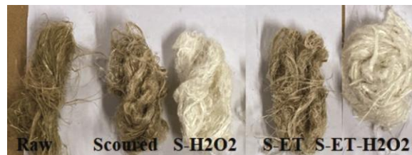
Fig. 8 — Raw, scoured, scoured-hydrogen peroxide bleached (S-H 2 O 2 ), scoured-enzyme treated (S-ET), and scoured-enzyme treated- hydrogen peroxide bleached (S-ET-H 2 O 2 ) flax fibres
