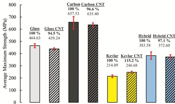
Fig. 6 — Average maximum flexural strength (MPa) data of the layered composites.
