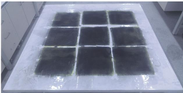
Fig. 1 — Kevlar fiber fabrics coated with CNT with a spray gun.
