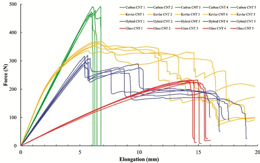
Fig. 11 — Three-point bending test results of layered composites with CNT additive.
