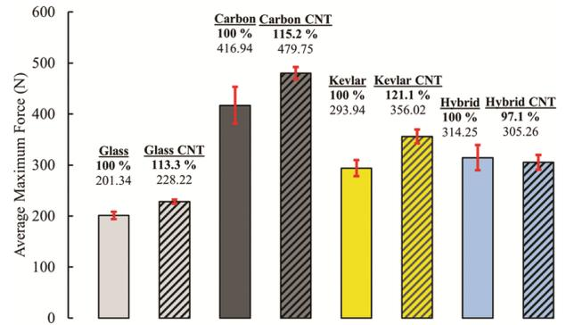
Fig. 7 — Average maximum force (N) data of the layered composites.
