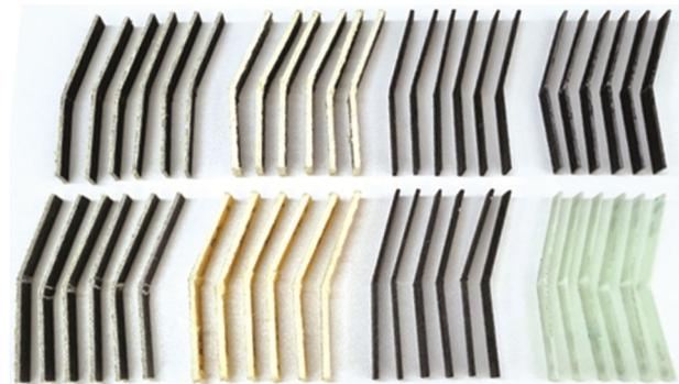
Fig. 5 — Three point bending test samples of layered composites after testing.
