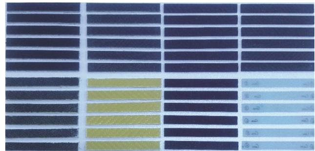
Fig. 3 — Tensile test samples produced in accordance with ASTM D7264 obtained from eight different composite plates.
