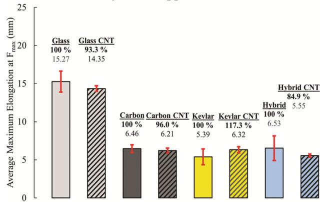
Fig. 9 — Average maximum elongation at critical failure (mm) data of the layered composites.
