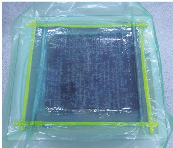
Fig. 2 — Composite plate that started to cure by applying the Vacuum Infusion production method.
