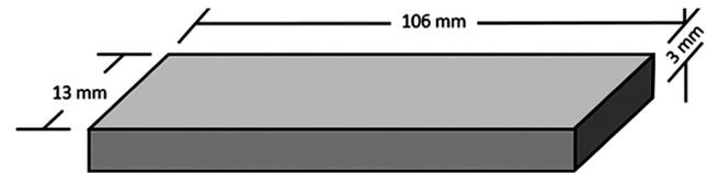
Fig. 4 — Dimensions of samples produced in accordance with the ASTM D7264 standard.
