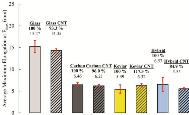
Fig. 8 — Average maximum elongation at maximum flexural force (mm) data of the layered composites.
