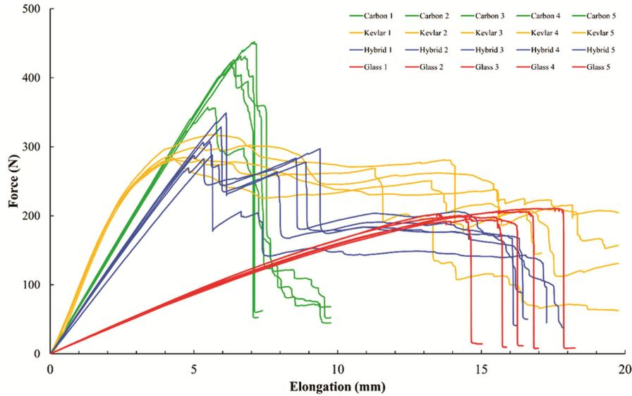
Fig. 10 — Three-point bending test results of layered composites.
