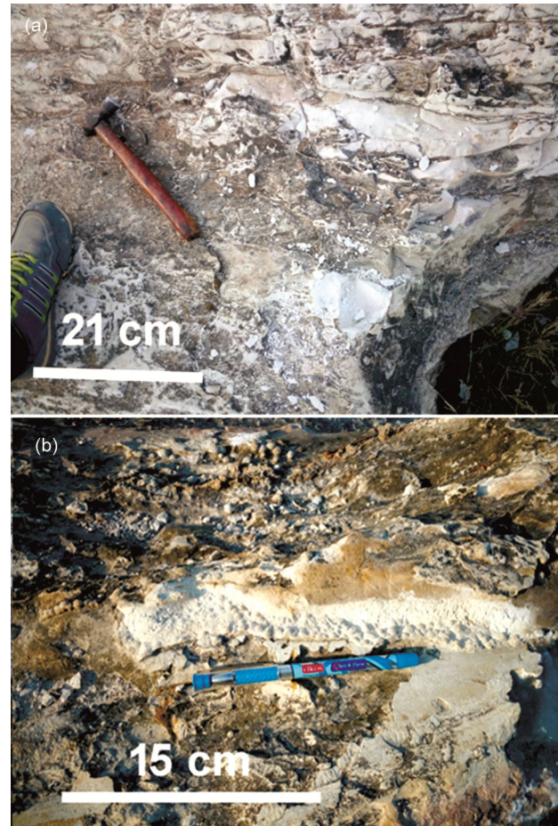
Fig. 5 — Optical photographs of (a) clay deposit, and (b) clay deposit showing presence of calcareous nodules.
