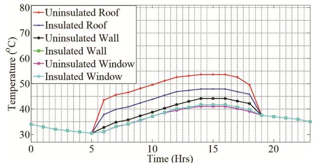
Fig. 3 — Solar air temperature for both test model.
