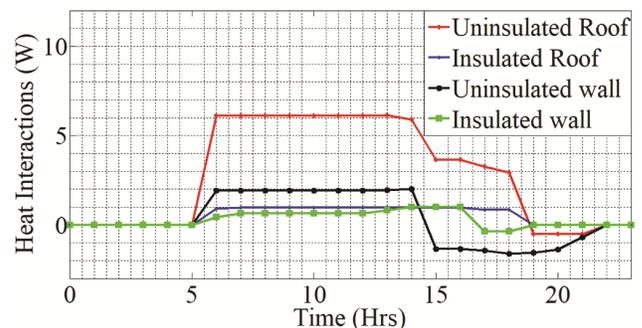
Fig. 4 — Heat interactions from roof and wall of test model without and with insulation.
