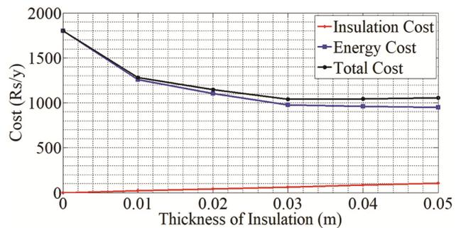
Fig. 9 — Optimum thickness of insulation.
