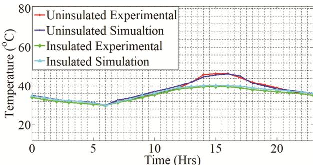
Fig. 8 — Simulated and experimental indoor temperature for uninsulated and insulated model.
