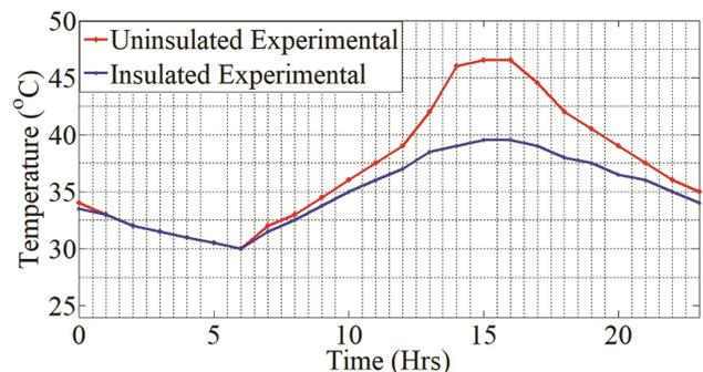
Fig. 7 — Experimental indoor temperature for insulated and uninsulated model.
