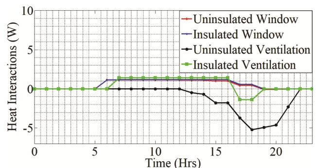
Fig. 5 — Heat interactions from window and ventilation for insulated and uninsulated model
