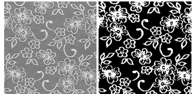
Fig. 5 — Original jacquard warp-knitted fabric image and pattern separation result by proposed method
