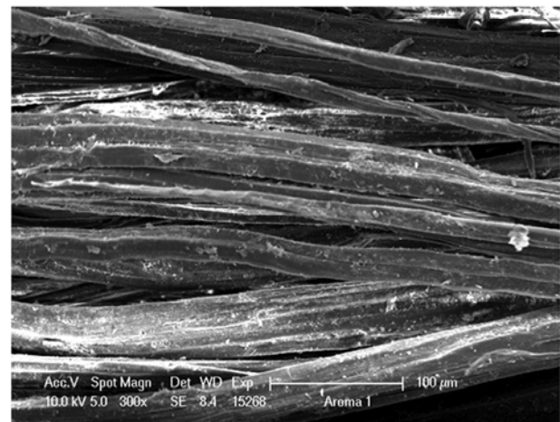
CHT:JO microcapsule applied jute fibre after 5 washes
