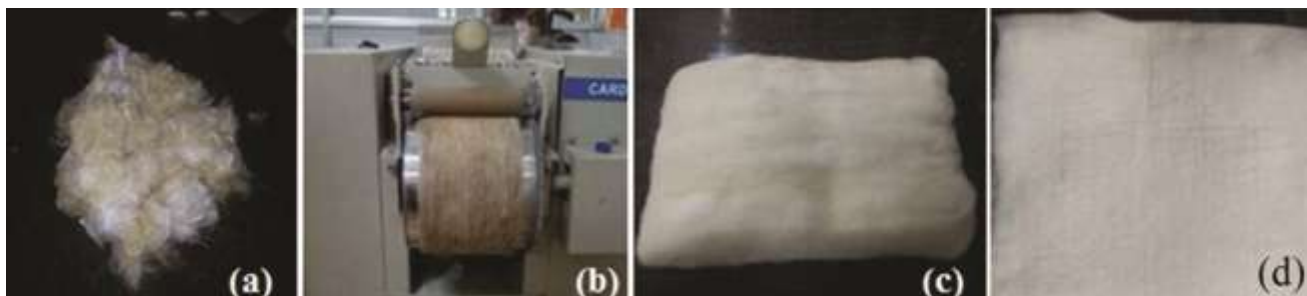
Fig. 1 — Carded web production (a) mixing of fibres, (b) web formation, (c) stacking of webs, and (d) needle-punched nonwoven fabric
