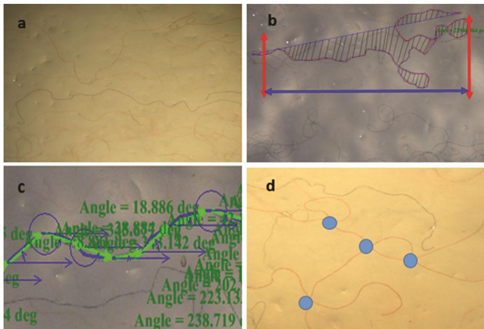
Fig. 1 — (a) Tracer fibre content – 0.3%, (b) fibre extent and area covered by fibre, (c) measurement of fibre inclination angle, and (d) cross-over point
