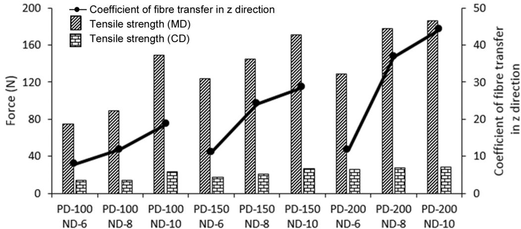
Fig. 6 — Relationship between tensile strength and coefficient of fibre transfer in Z direction
