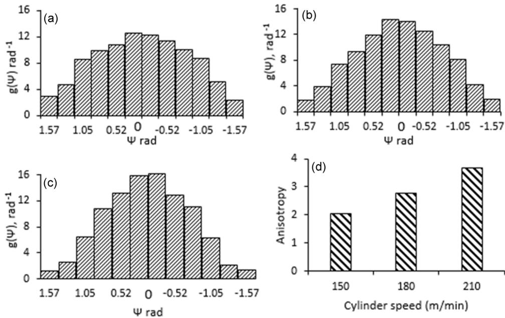
Fig. 3 — Distribution of fibre orientation at different cylinder speed (a)150m/min, (b) 180m/min and (c) 210m/min, and (d) anisotropy of all three fibre webs
