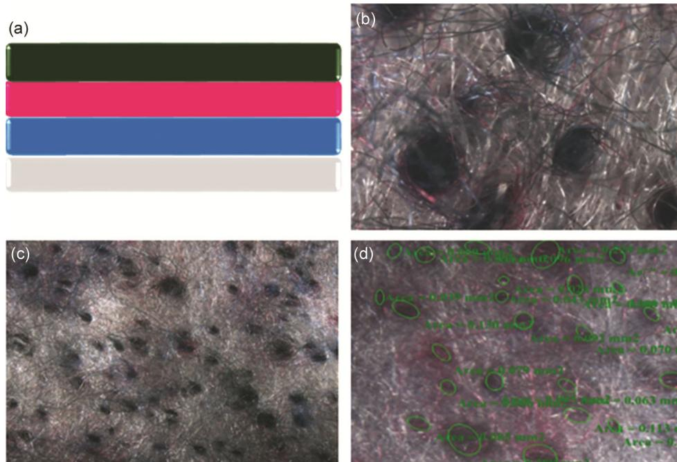
Fig. 2 — (a) Layering sequence of layers, (b) presence of different colours on bottom most layer after punching, (c) number of holes and (d) area covered by the holes
