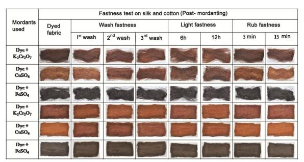
Fig. 4 — Silk and cotton fabrics dyed with M. suriga dye along with chemical mordants and fastness tests (post-mordanting)
