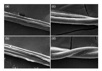
Fig. 5 — SEM images showing the surface morphology (a) raw silk fibre (b) silk fibre dyed with *M. suriga* dye extract (c) undyed cotton fibre and (d) cotton fibre dyed with *M. suriga* dye extract [x1000]
