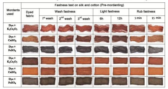
Fig. 2 — Silk and cotton fabrics dyed with M. suriga dye along with chemical mordants and fastness tests (pre-mordanting)
