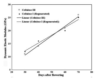
Fig. 4 — Relationship between dynamic elastic modulus and maturity of cellulose III and cellulose I(regenerated)
