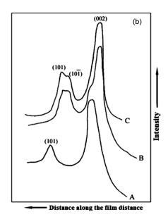
Fig. 2 — X-ray diffractograms of (a) cellulose I [(A) untreated, (B) after 2h of treatment, and (C) after 4h of treatment; and (b) cellulose III [(A) untreated, (B) after 15 h of treatment and (C) after 24 h of treatment
