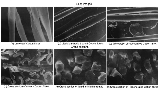
Fig. 1 — Scanning electron micrographs (×640) of (a) untreated, (b) liquid ammonia treated and (c) regenerated; and cross-sections of the (d) untreated mature, (e) liquid ammonia treated and (f) regenerated cellulose 1 fibres respectively.
