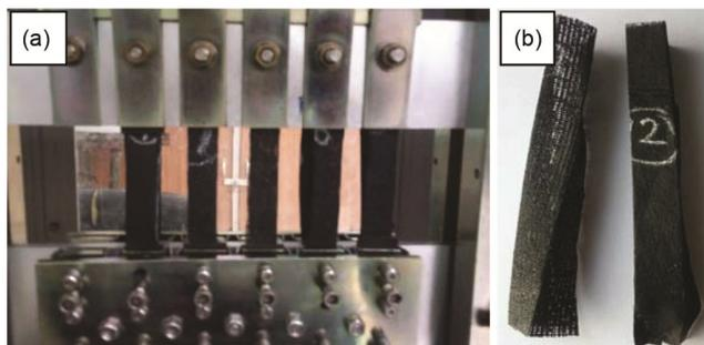
Fig. 5 — (a) Samples mounted in Dematia Flex Tester, and (b) tested sample of coated fabric
