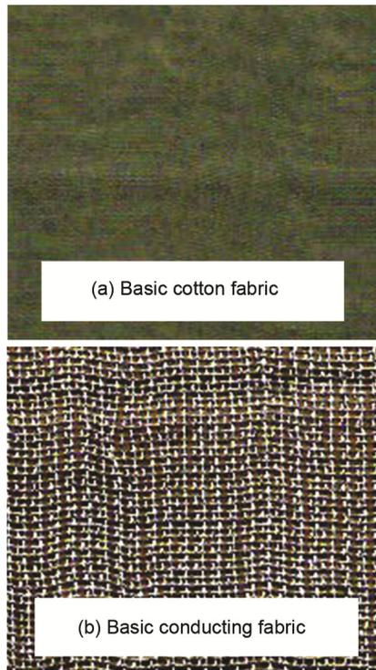
Fig. 1 — Visual image of (a) basic non- conducting cotton fabric and (b) basic conducting fabric
