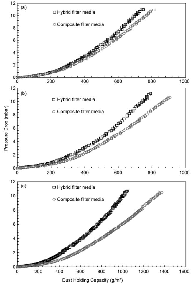
Fig. 3 — Evolution of pressure drop with dynamic loading of dust in case of composite filter media and hybrid filter media: (a) equal proportion of 19.13  $\mu\text{m}$  and 30.17  $\mu\text{m}$  fibres, (b) equal proportion of 19.13  $\mu\text{m}$  and 48.24  $\mu\text{m}$  fibres and (c) equal proportion of 19.13  $\mu\text{m}$ , 30.17  $\mu\text{m}$ , and 48.24  $\mu\text{m}$  fibres
