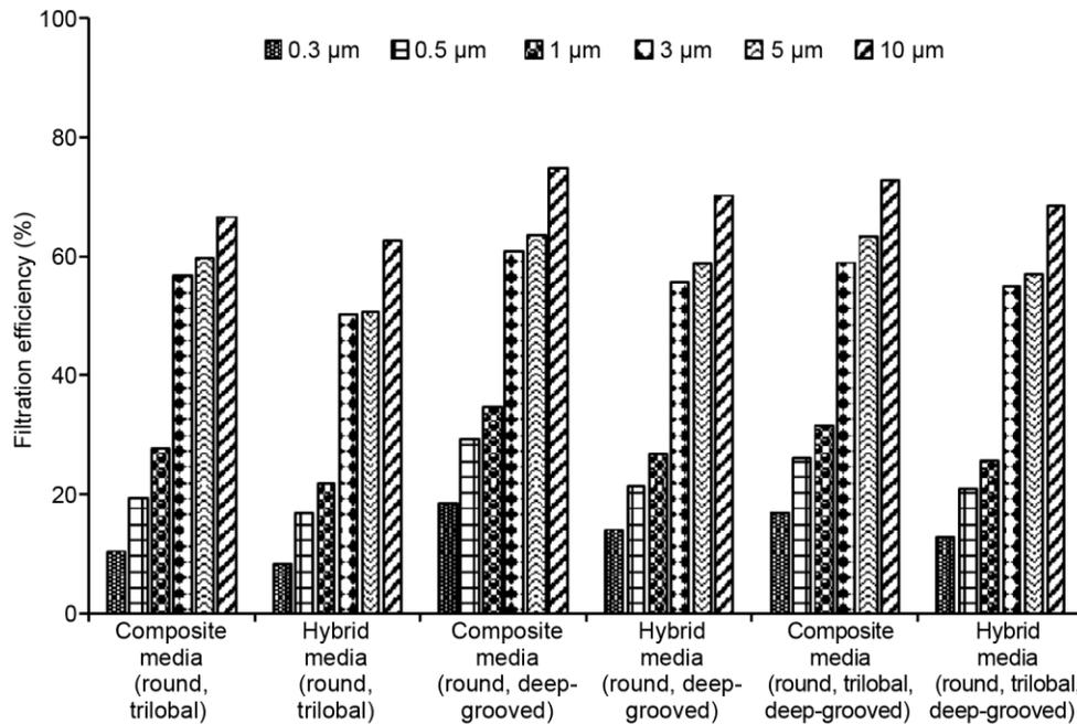
Fig. 5 — Comparison of filtration efficiency of composite filter media and hybrid filter media made up of fibres of different shapes
