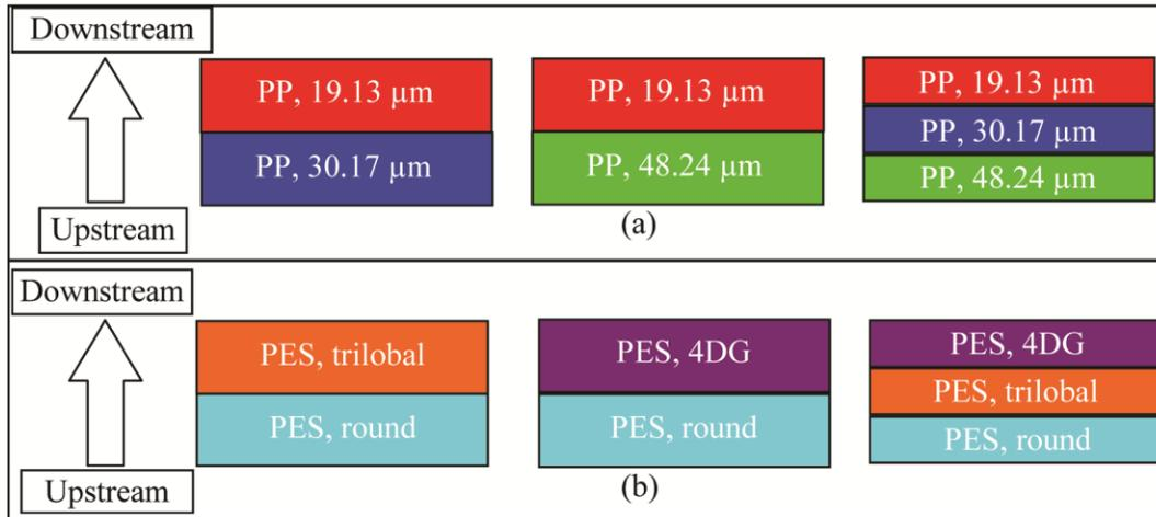
Fig. 1 — Schematic diagram of nonwoven filter media with hierarchically arranged fibres of different sizes (a), and shapes (b)
