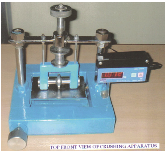
Fig. 1 — Photograph of fibre crushing instrument 6
