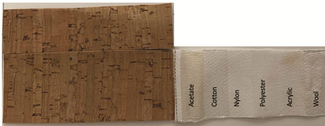
Fig. 4 — Color fastness test result of knitted backed cork leather
