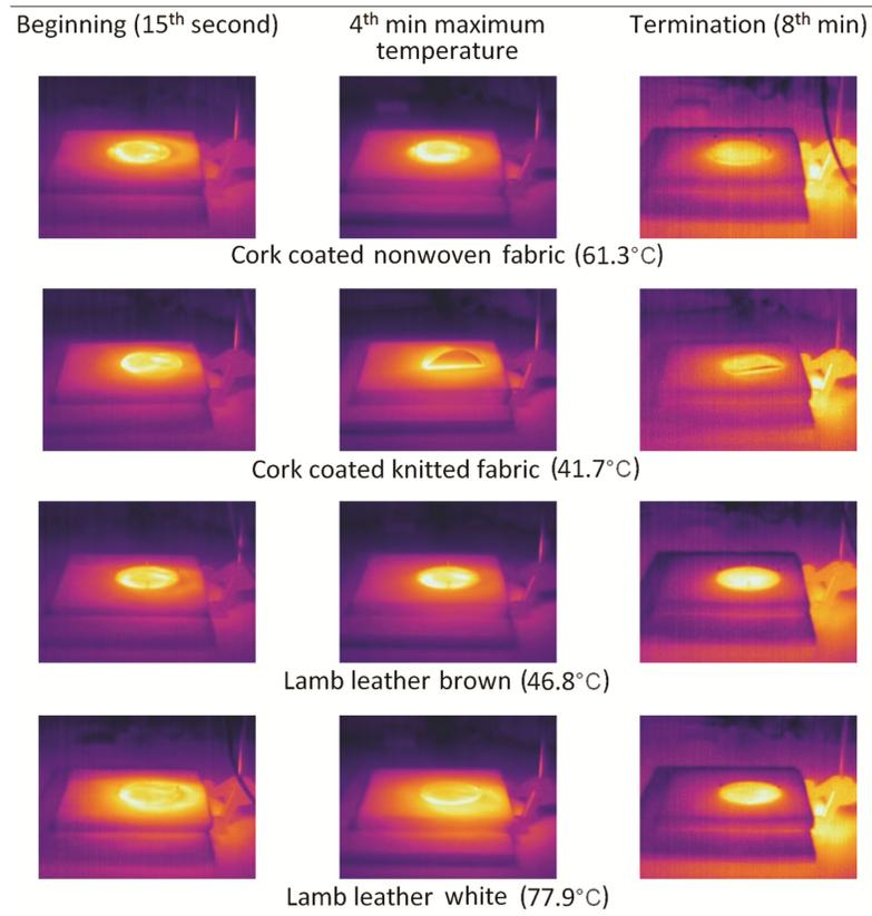
Fig. 6 — Thermograms with measured temperature of all investigated leather, recorded with thermal imaging camera
