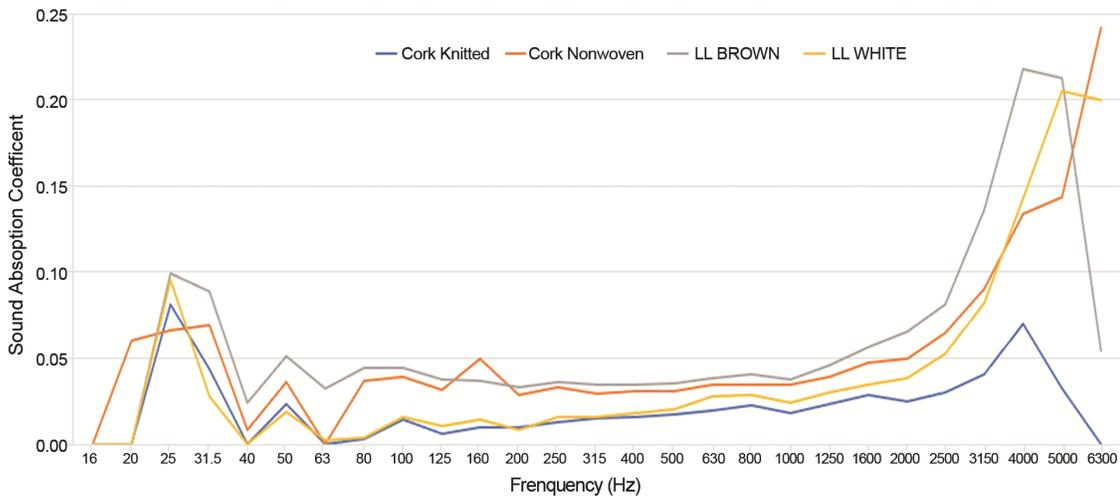
Fig. 5 — Sound absorption properties
