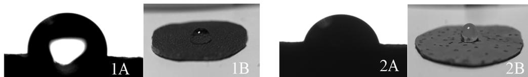
Fig. 3 — 1A/1B- lamb leather brown contact angle and 2A/2B- cork coated knitted fabric contact angle
