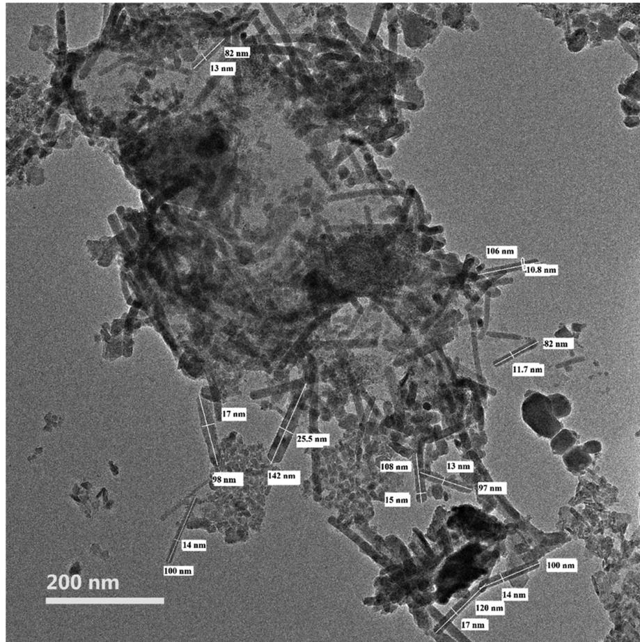
Fig. 3 — TEM image of banana cellulose nano-crystal
