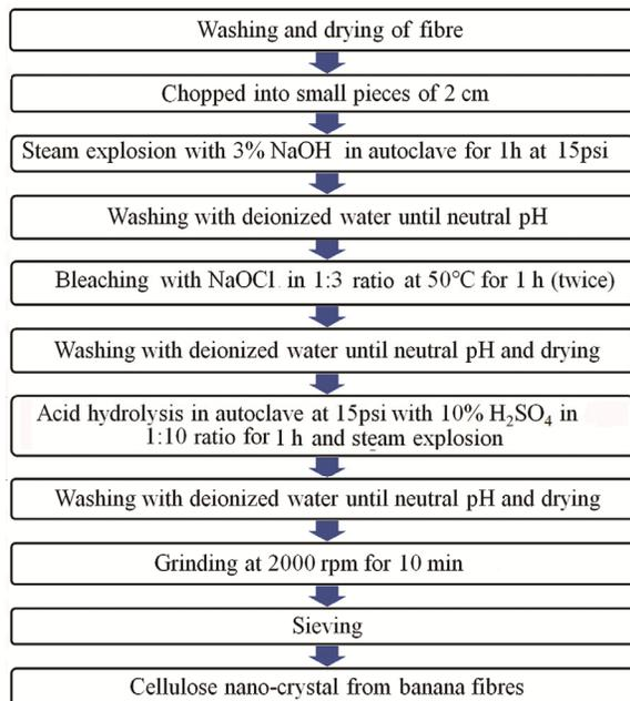
Fig. 1 — Extraction process of cellulose nano-crystal from banana fibres
