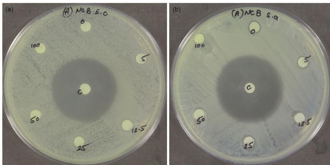
Fig. 7 — Antibacterial analysis of banana cellulose nano-crystal against bacteria (a) *E. coli* and (b) *S. aureus*
