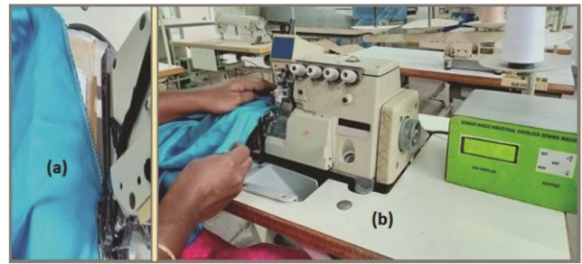
Fig. 6 — (a) Over-lock stitch formation and (b) sewing garment using flex touch sensor method
