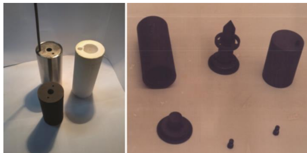
Fig. 1 — Structure of copper point blackbody cavity.
