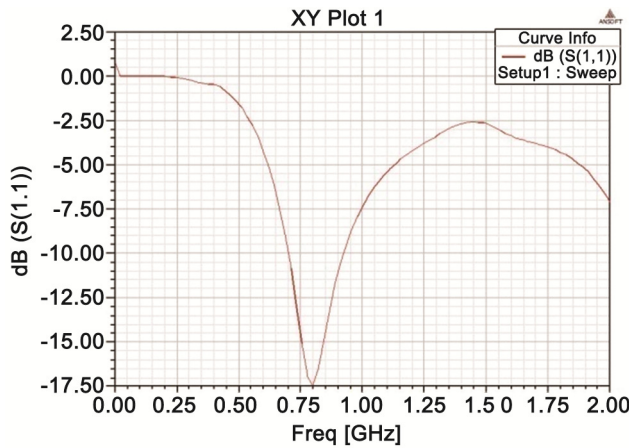
Fig. 11 — S-parameter for plasma antenna of radius 1.5 cm and length 10 cm.
