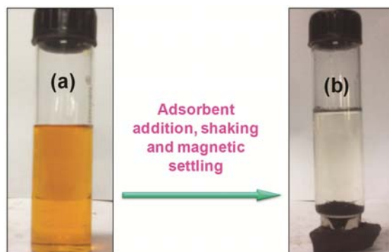
Fig. 11 – Adsorption of methyl orange (MO) dye using Fe_3O_4@AC NC containing ~22 wt % of oleic acid capped Fe_3O_4 nanoparticles (FAC4) followed by magnetic separation of spent adsorbent particles.
