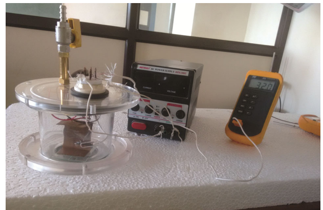
Fig. 2 — Experimental setup for calculation of thermoelectric power.
