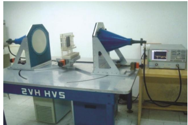
Fig. 3 — Experimental arrangement for microwave measurement
