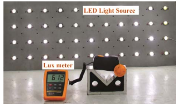
Fig. 13 — Linearity measurement by Lux meter setup.
