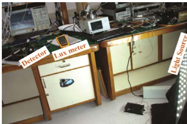
Fig. 15 — Linearity measurement by detector setup.
