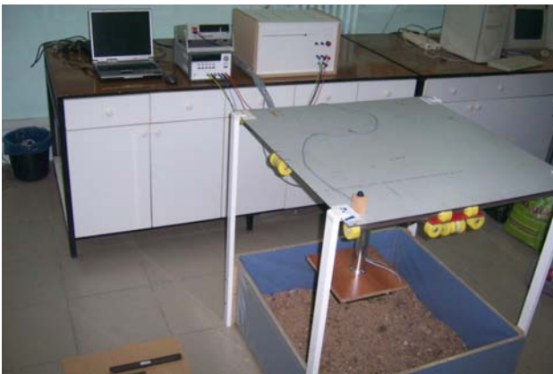
Fig. 9 — Test bed of the magnetic measurement system
