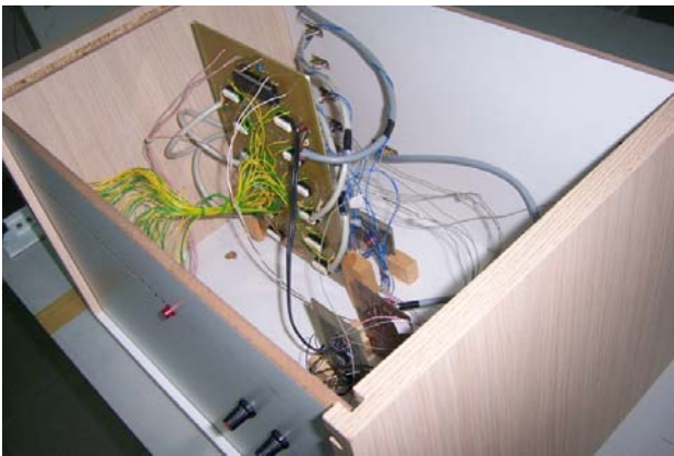
Fig. 4 — Electronic control unit of the magnetic measurement system developed here
