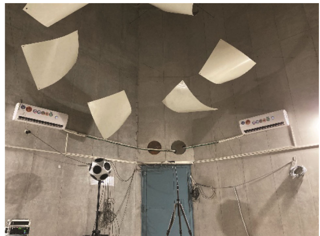
Fig. 2 — Reverberation chamber facility at CSIR-National Physical Laboratory, New Delhi.
