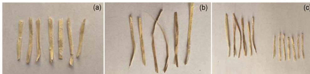
Fig. 10 — (a) Vetiver grass fiber of length 30-40 mm (b) Vetiver grass fiber of length 60-70 mm (c) Vetiver grass fiber of length 30-40 mm and 60-70 mm.
