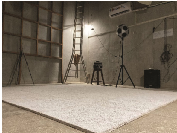
Fig. 5 — Vetiver grass panel of density 400 kg/m 3 and thickness 20 mm installed in a reverberation chamber at rigid surface backing at CSIR-National Physical Laboratory, New Delhi.
