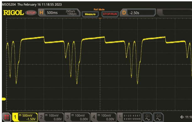
Fig. 5 — Unprocessed absorption spectrum from chip-scale vapour cell observed on oscilloscope.
