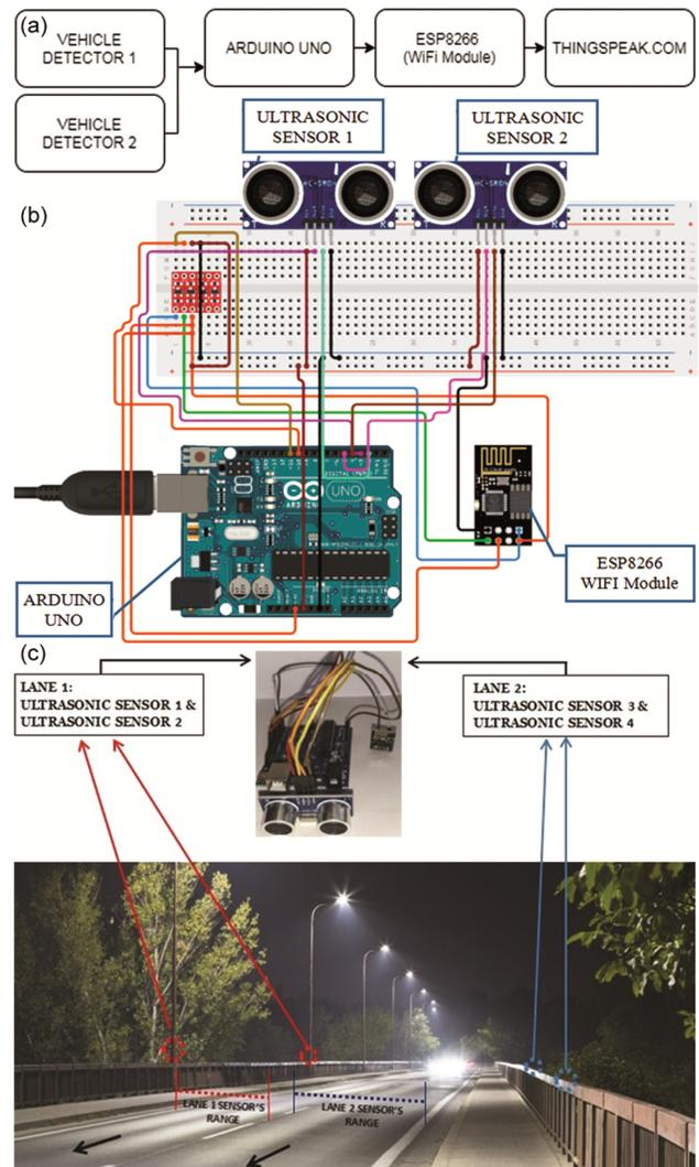
Fig. 1 — (a) Block diagram of the proposed system, (b) circuit connections of the proposed system, and (c) proposed experiment set up placement in a two-lane road.
