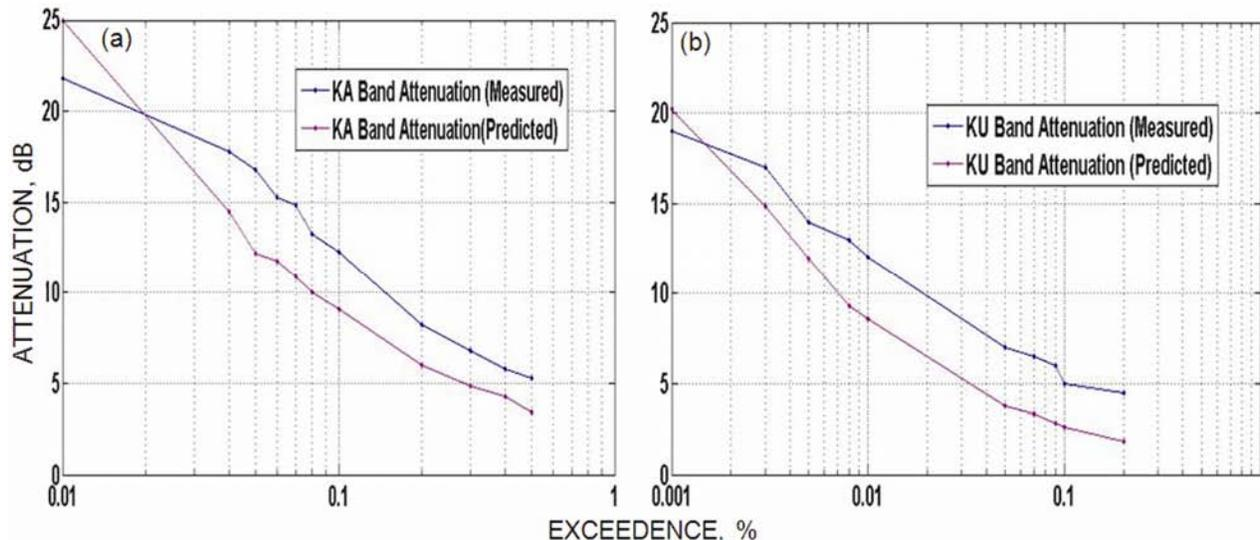
Fig. 3 — Comparative plot of attenuation exceedance derived from the model and measurement for: (a) Ka band; and (b) Ku band
