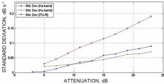
Fig. 5 — Variation of the standard deviation of the fade slope distribution with base attenuation
