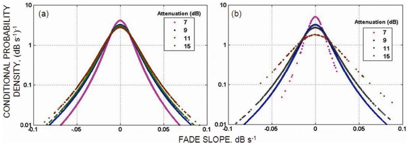
Fig. 4 — Conditional fade slope distributions for: (a) Ka band; and (b) Ku band
