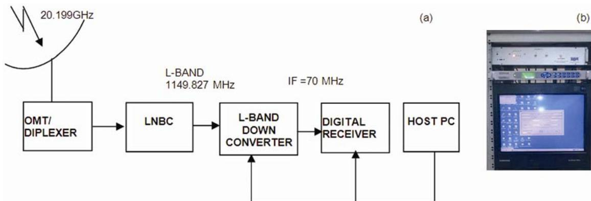
Fig. 1 — (a) Schematic for the set up of the Ka and Ku band beacon receivers at Delhi Erath Station; and (b) Integrated set up
