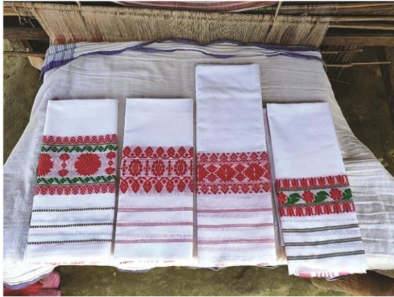
Fig. 4 — Bihuwan yarn specification: 2/60s mercerised white, red and green cotton for warp, weft, and motifs s. Yarn procured from Kumar Stores, Guwahati. Textile woven by weaver Ms. Rubi Bora under the supervision of UGC STRIDE Master Weaver Ms. Dipti Das Bhuyan in Nameri, Sonitpur district, Assam. Weave pattern: Plain weave
