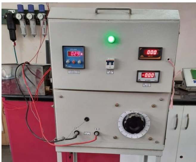
Figure 1: CHF measuring Instrument (A) Schematic diagram of instrument set-up; (B) Real-time image of the instrument
