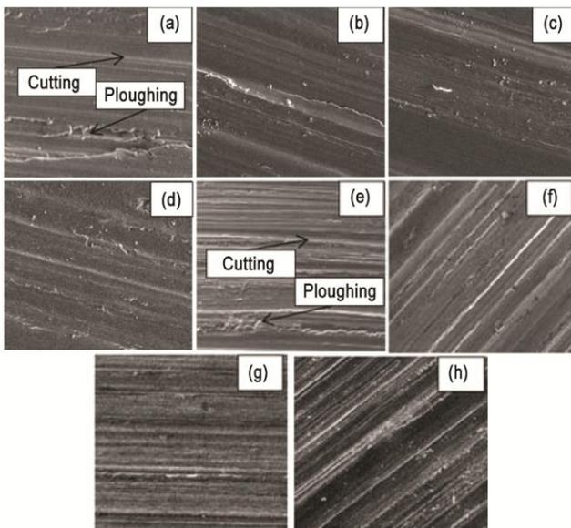
Fig. 6 — Worn surface images of fabricated composites for the load and sliding distance of (a) 20 N and 300 m, (b) 30 N and 300 m, (c) 20 N and 500 m, (d) 30 N and 500 m, (e) 20 N and 300 m, (f) 30 N and 300 m, (g) 20 N and 500 m, (h) 30 N and 500 m at 500 x.
