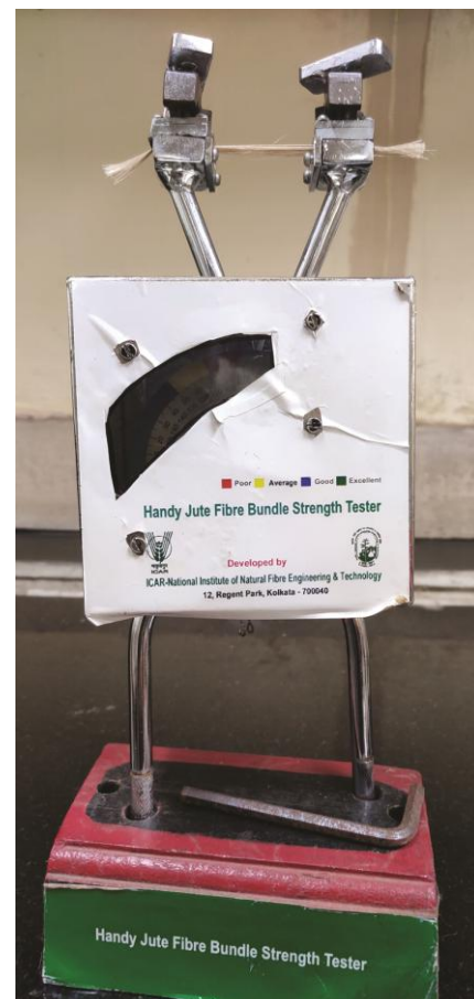
Fig. 2 — Prototype of the developed bundle strength tester
