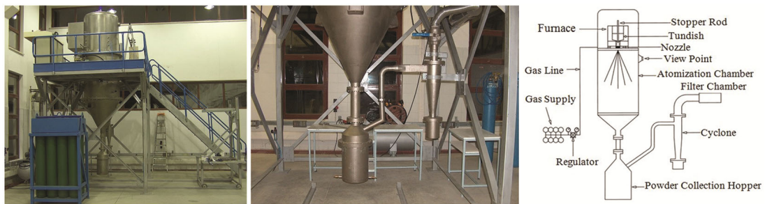
Fig. 2 — Detail of gas atomization unit
