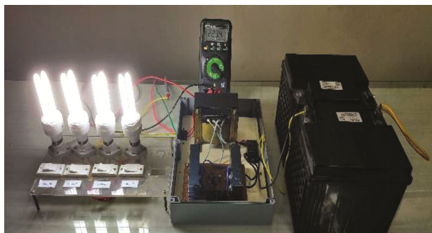
Fig. 6 — Inverter supplying power to the load
