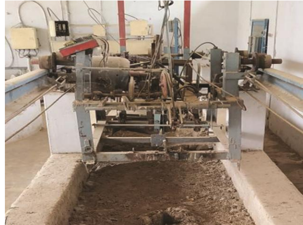
Fig. 2 — Linear Soil bin
