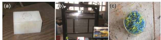
Fig. 3 — Different components of model tank: (a) Model Strip Footing, (b) Model Tank, (c) Fibers
